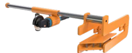
The Groove Tool reduces yaw brake noise, by cutting grooves in the yaw brake disc, which acts like a razor as the turbine moves to meet the wind, cutting debris from the brake pad.
