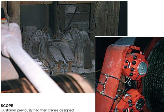
Customer previously had their cranes designed with electro magnetic brakes but after only a few years on hot metal cranes they mal-functioned.
