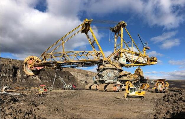
**Image 1:** Bucket wheel excavators (BWEs) need robust and reliable braking systems to withstand the harsh operating and environmental conditions they are exposed to.
